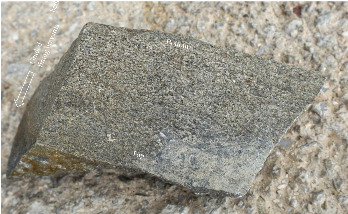
Outcrop X. Silty limestone from kink band indicating graded bedding and deposition by turbidity flow
