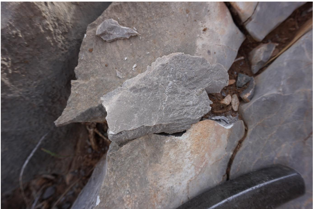
Outcrop XIII. Sample of the limestone shown in the previous picture. Notice that the limestone has not undergone significant metamorphism (as it is not marble) and therefore cannot be part of the Asterousia crystalline nappe.
